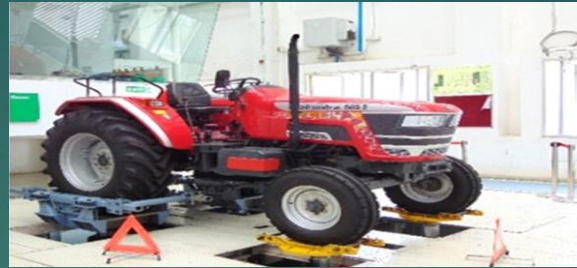
Three Poster Tractor Test Facility
